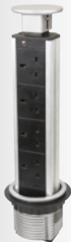
Item No.509108-B UK Sockets 4 ways 240V, 13A Size: Ø 90x367mm
