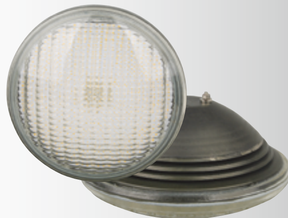
Item No.403024 Rating Power: 53W 12V.AC. PAR56,240xSMD Beam Angle: 120° Light Color: CW/WW/BE/RGB Lumen: 3200LM
