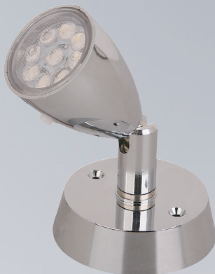
Item No.:202796-B Lumen:55LM 12VDC,0.8W 9LEDs*SMD3528 Diamond lense Total length:90mm Material: Plastic, metal With switch
