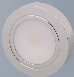
Item No.:202778-I Lumen:250LM 12VDC,3.6W 9xLEDs*SMD2835 Size:Ø65*10mm Material: Alum, Plastic
